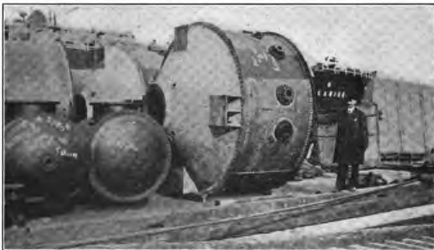
FIG. 143.—Lower section of a vacuum pan for export to Formosa, 11 ft. diam. \times 8 ft. 6 in. long, with calandria inside, gross weight 19,400 lb.; shell of steel, bottom of cast iron: flanges should have been protected.
